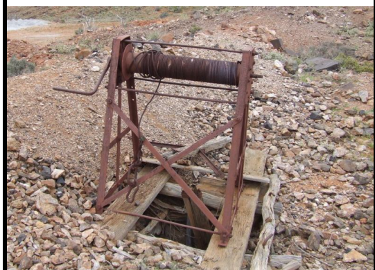
Below: Old hand windlass over the south shaft at Freyer's Wolfram Mine.
